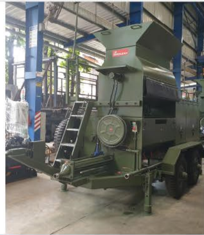
Rapid Runway Repair Vehicle
